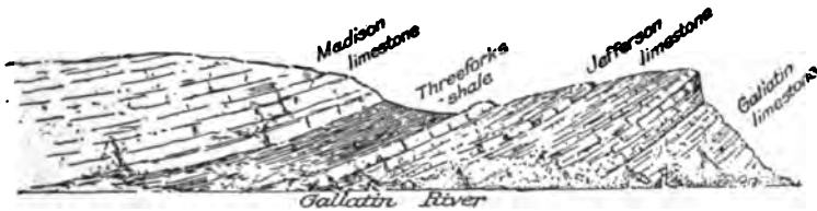
FIG. 1356. — Section on the Gallatin River near Logan, Mont., showing the Madison limestone (Mississippian) resting with apparent conformity upon Devonian (Three Forks shale and Jefferson limestone), which in turn rests disconformably upon the Cambro-Ordovician Gallatin limestone. (U. S. G. S.)
